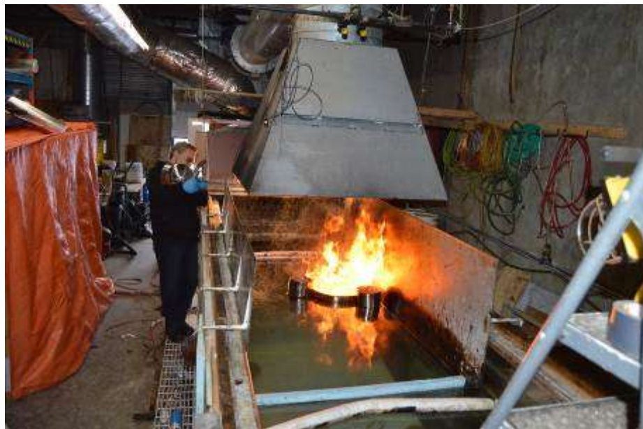
Figure 8: Wind/wave tank set up for burn experiments with heat shields and exhaust hood.
