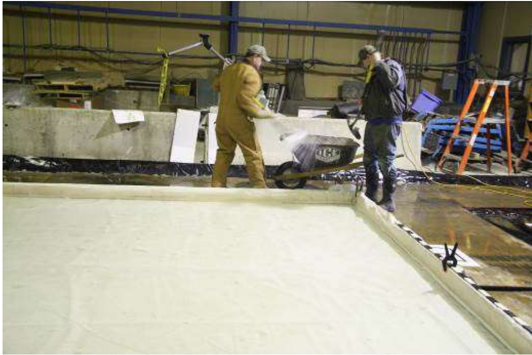
Figure 28: Shovelling loose natural snow onto the water surface to create slush ice.
