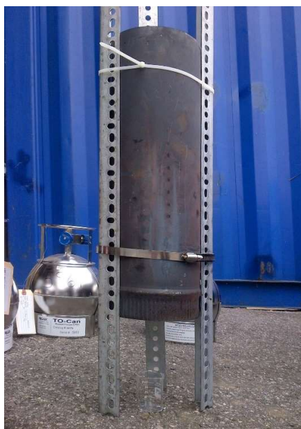
Figure 93: Stack assembly used in Herder/Torch Impingement tests
