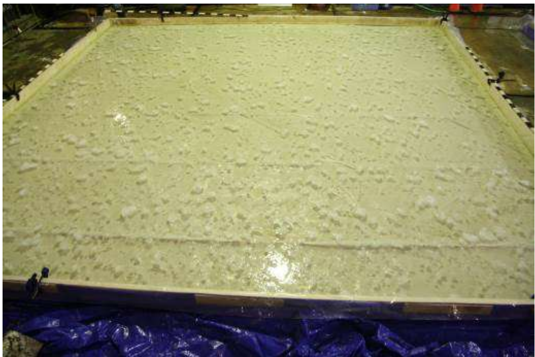
Figure 27: Test pool filled with salt water with slush ice.
