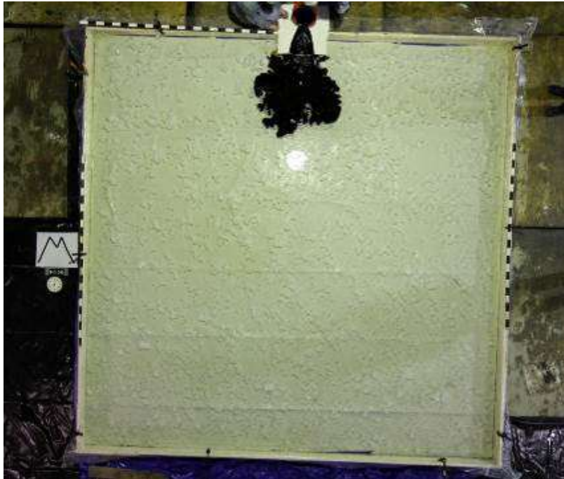
Figure 31: Pouring oil onto water on test pool at start of test.
