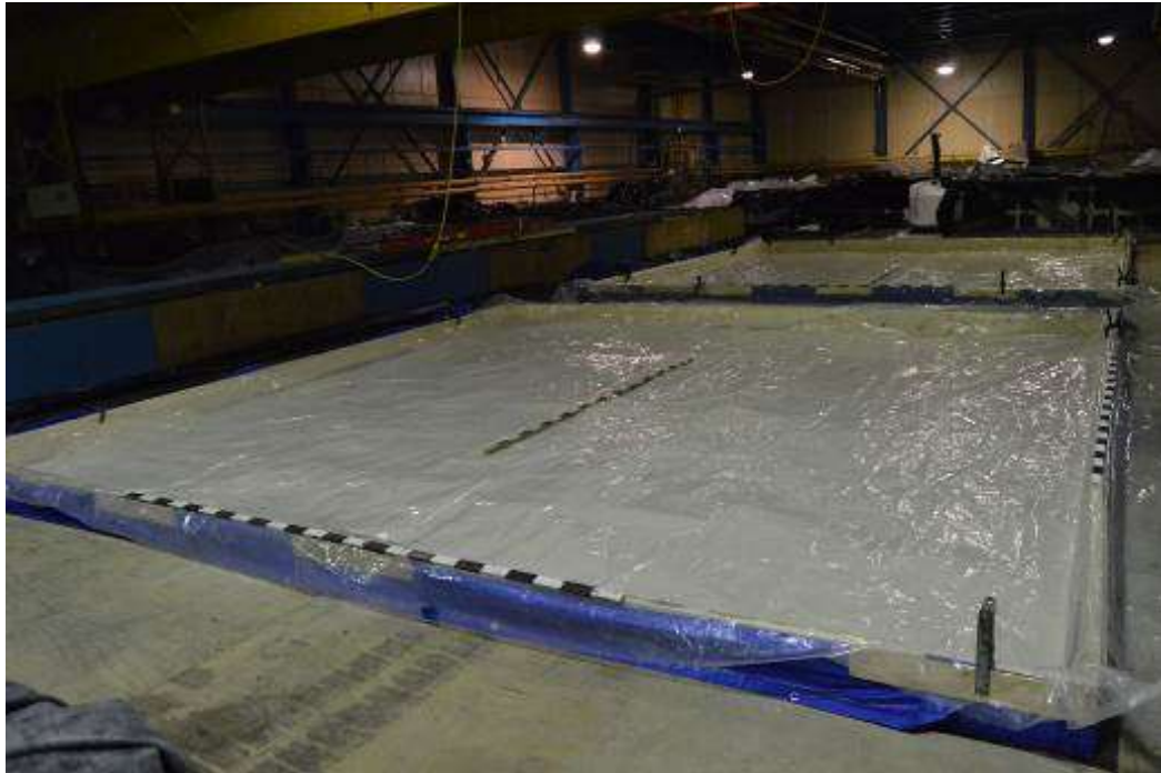
Figure 26: Lined test pools on sand in Research Area at CRREL.
