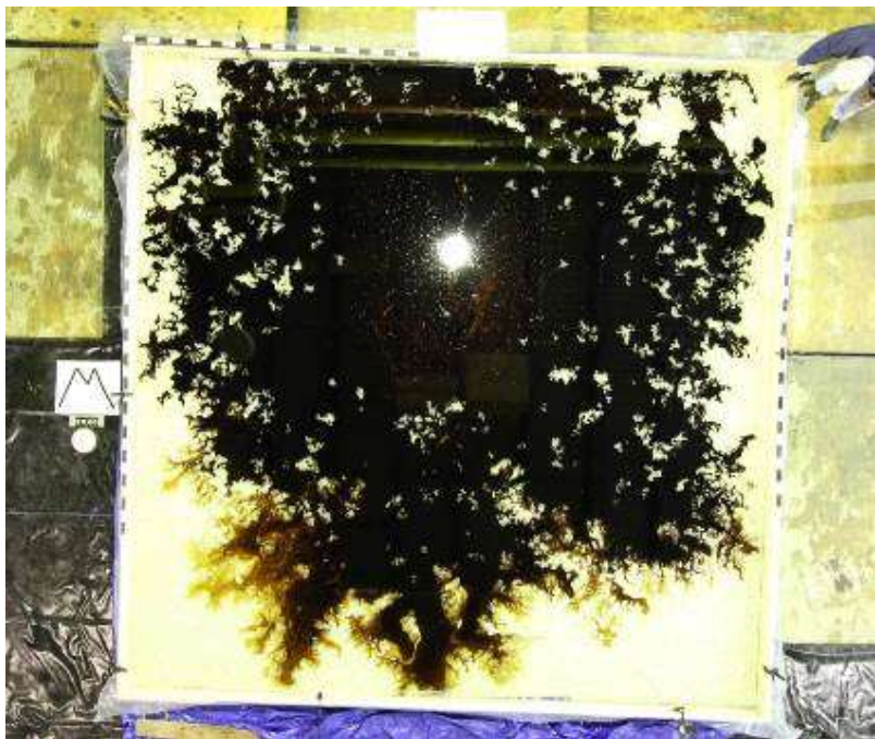
Figure 32: Oil spread to equilibrium thickness in slush ice.
