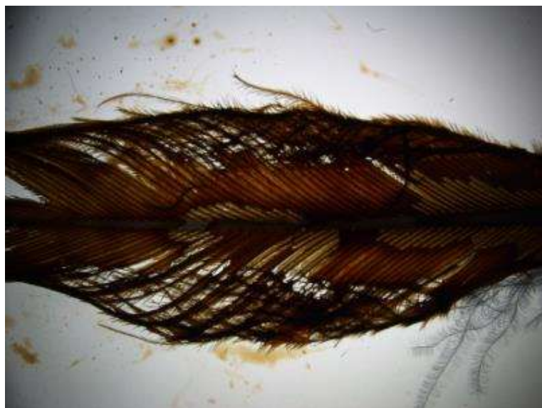
Figure 85: Example of a feather heavily smeared in oil, thus AI is set to 25. Thick-billed Murre exposed to TS6535 and ANS (1.16 \mu\text{m} ; estimated sample thickness based on the assumption that the oil sample was homogeneously distributed over the test surface area, however note that the oil was herder and probably much thicker).
