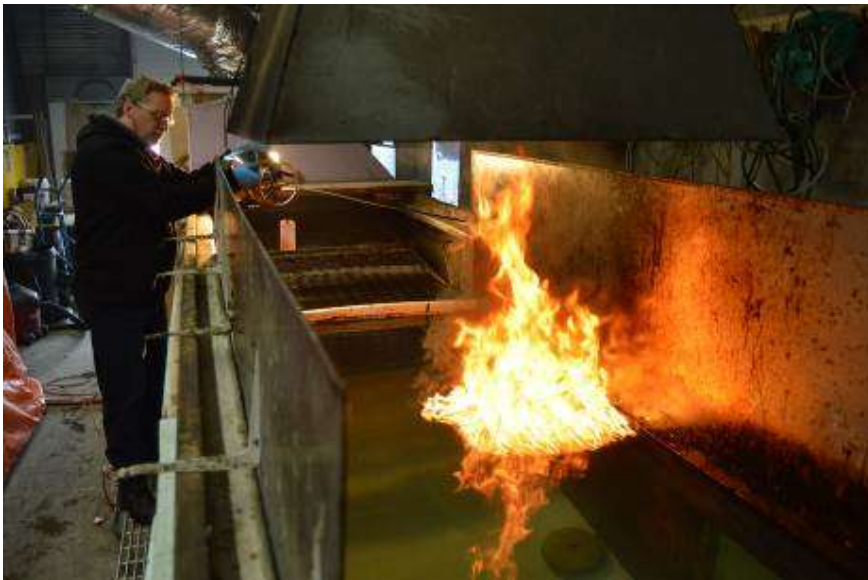
Figure 6: Herded slick burning under fume hood suspended over wind/wave tank.
