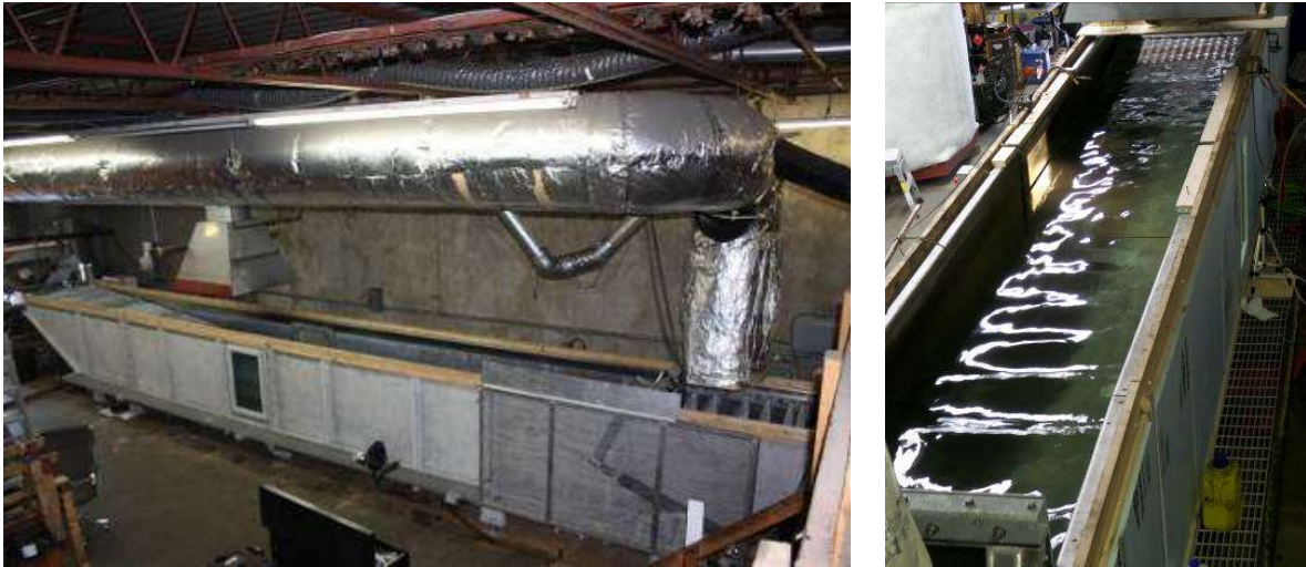
Figure 5: New aluminium wind wave tank in SL Ross laboratory.
