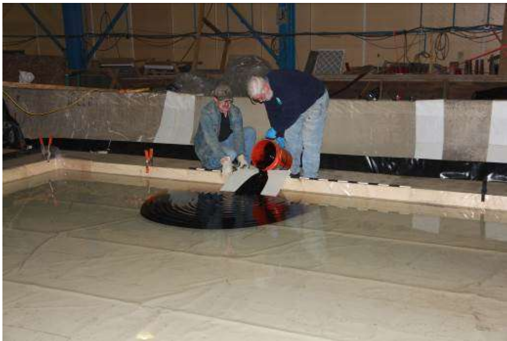
Figure 29: Pouring crude oil from bucket down spill plate onto water surface.
