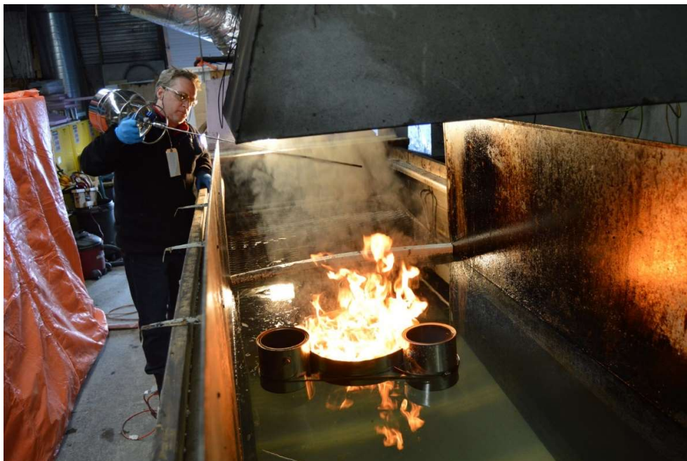
Figure 91: Mechanically contained oil burning
